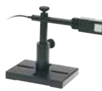
PD300 with filter installed
