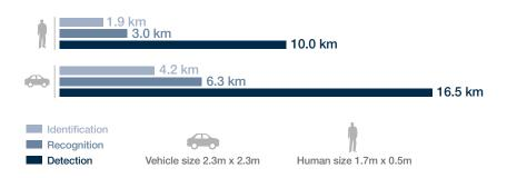
Assumptions: detector  $10\mu$  pixel pitch |  $3.6\mu$ - $4.9\mu$  spectral band | 23mK NETD| 30Hz frame rate|  $0.2km^{-1}$  atmospheric attenuation coefficient | 50% detection probability | 1.7x0.46m human size | 2.3x2.3m vehicle size
